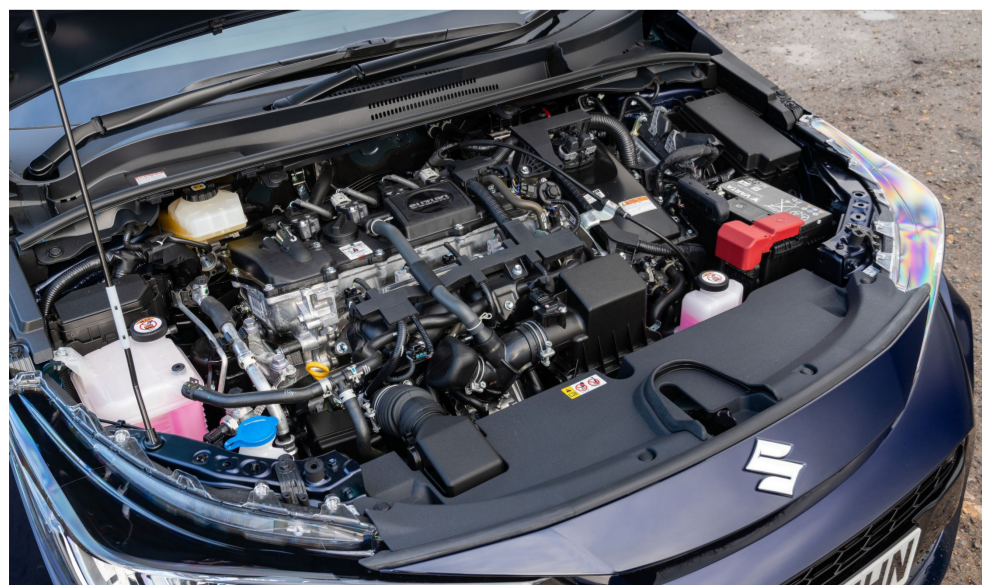
■ The Swace is powered by a 1.8-litre petrol engine joined with a small electric motor
